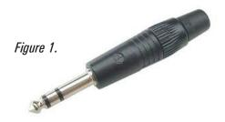
Figure 1. shows a TRS connector with the three conductors separated by the black insulation bands. The pointed front of the connector is the tip, the middle band is the ring, and the large conductor at the rear nearest the plug body is the sleeve.
